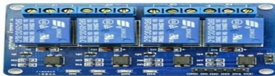
**Gambar 2.8** Relay 4 Channel
