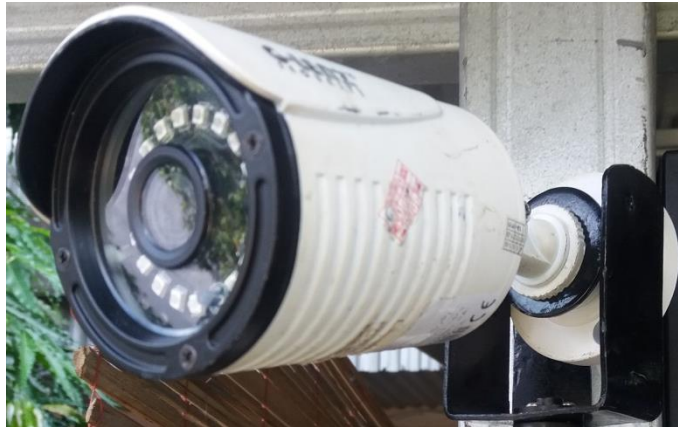
Gambar 2.1 CCTV ( Closed Circuit Television )
