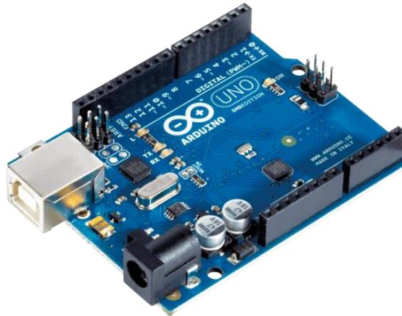
**Gambar 2.1 Board Arduino Uno**
