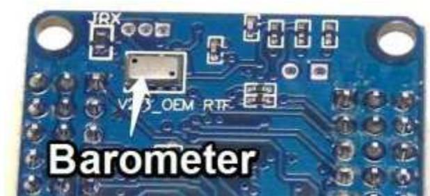
Gambar 2.19 Barometer
