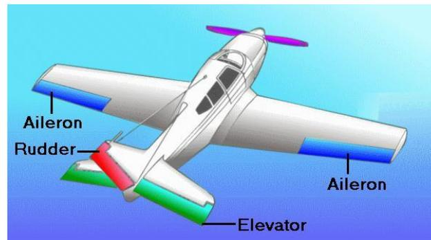
Gambar 2.9 *Primary flight control surfaces*
