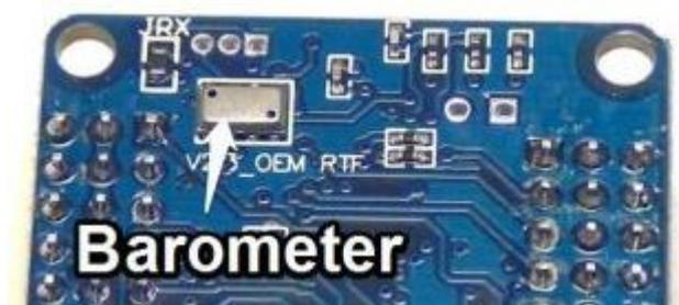
Gambar 2.19 Barometer
