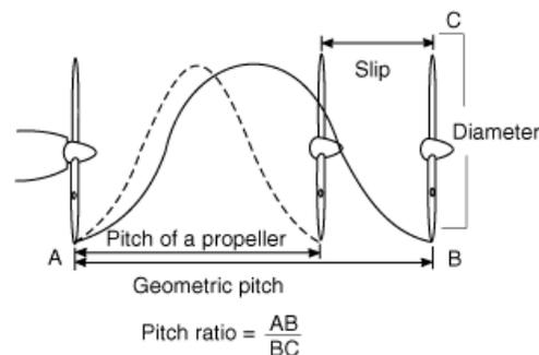
Gambar 2.10 *Pitch of Propeller*
