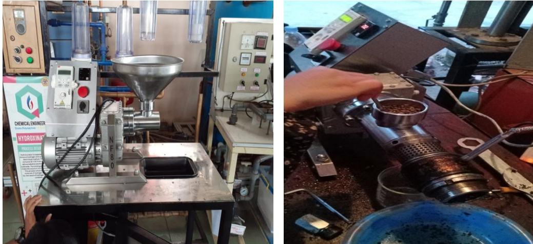
Gambar III.1 Alat Screw Oil Press Machine dan Proses Pengepresan Biji Kapuk
