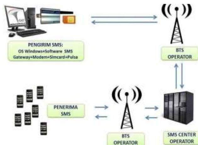
**Gambar 2.2** Blok Diagram SMS Gateway
