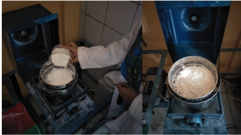
Gambar 11. Tepung diayak di vibrating screen
