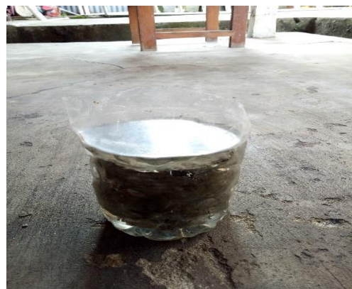
Gambar C.16. Perendaman Sampel (Pengujian Daya Serap)
