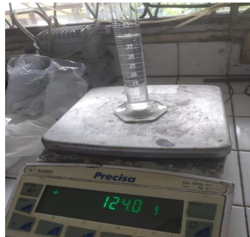
Gambar C.14. Penimbangan Gelas Ukur+Aquadest (Pengujian Densitas)
