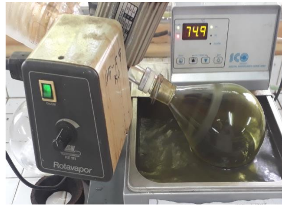
Proses Rotavapor ( Rotary Vacuum Evaporator )
