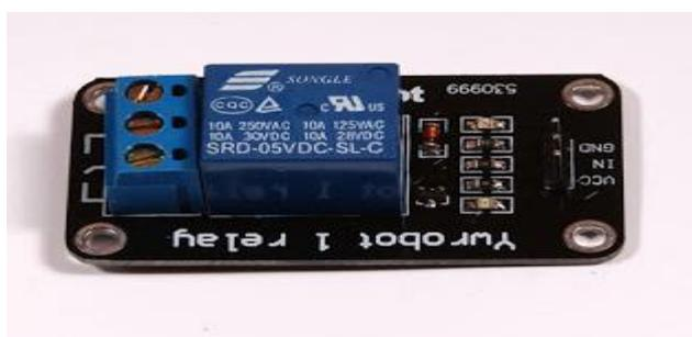
**Gambar 2. 14** Module Relay 1 Channel
