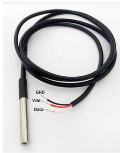
Gambar 2.14 Sensor Suhu DS18B20 (Pakpahan Feri, 2018)
