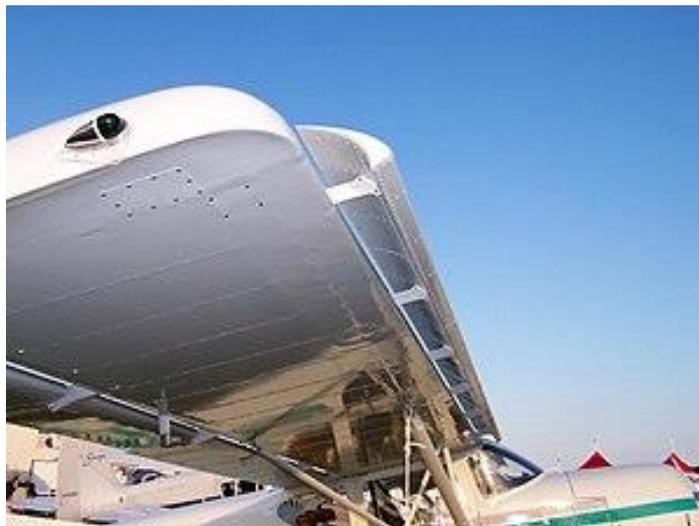
**Gambar 2.6** *Aircraft Slat (GMF Module Structure, 2016)*
