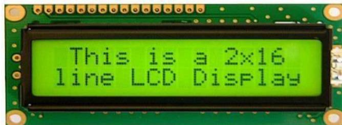
**Gambar 2.13** Liquid Crystal Display
