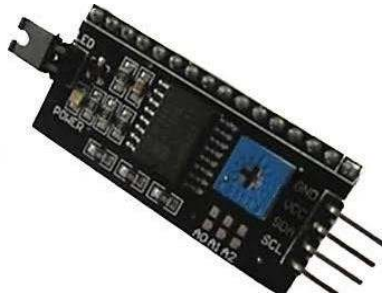
Gambar 2.17 LCD Modul I2C (Khoirul Iman, 2016)
