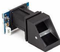
Gambar 2.5. Modul sensor sidik jari R305 (Rhydolabz,2014)
