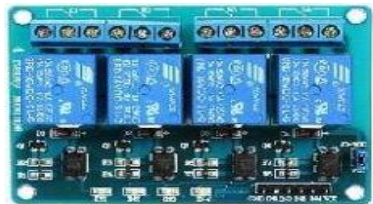
Gambar 2.21. Modul Relay 4 beban (Henry Bench, 2016)
