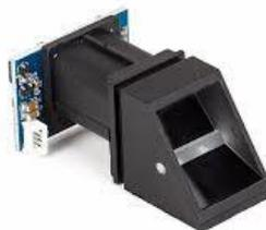
Gambar 2.5. Modul sensor sidik jari R305 (Rhydolabz,2014)
