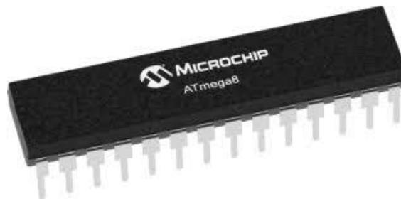
**Gambar 2.9** Mikrokontroler ATmega8 (Ragil Ahyanto,2017)
