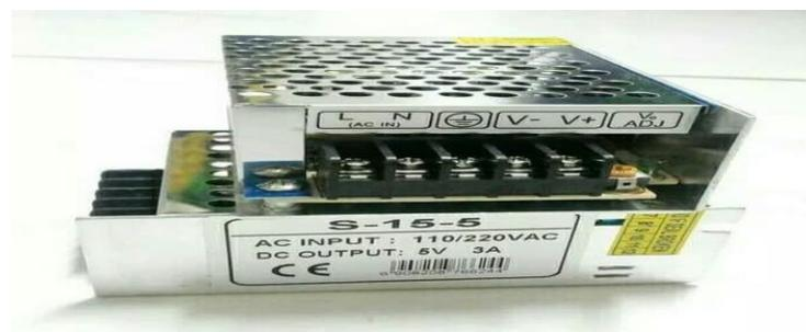
Gambar 2.14: Power Supply 5 V 3 A
