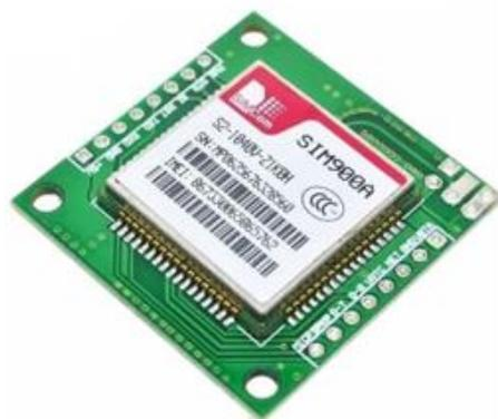
**Gambar 2.14** Modul GSM SIM900A
