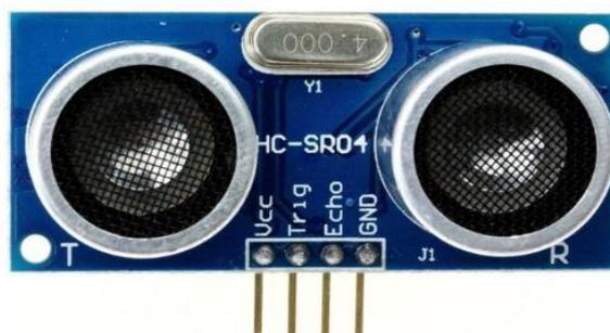
**Gambar 2.6** Sensor Ultrasonik HC-SR04
