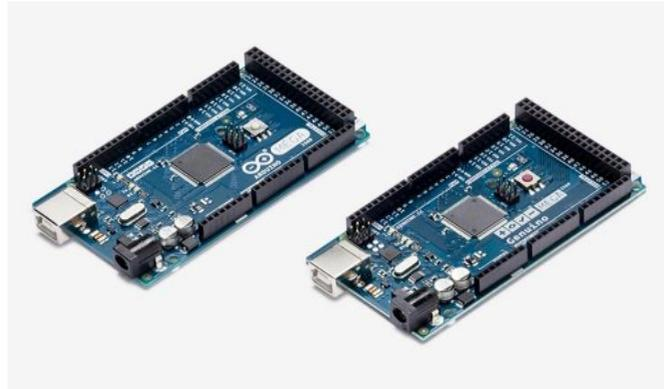
**Gambar 2.7** Arduino Mega 2560
