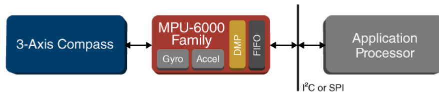
Gambar 2. 6 Diagram Modul MPU-6050
