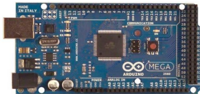
Gambar 2. 7 Arduino Mega 2650 (Sumber : ArduinoMega2560Datasheet.pdf )
