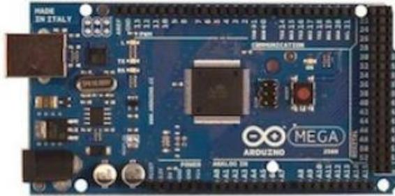
**Gambar 2.12** Arduino Mega
