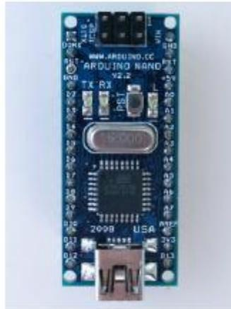
**Gambar 2.16** Arduino Mini/nano
