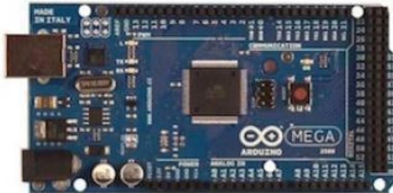
**Gambar 2.17** Arduino Mega 2560
