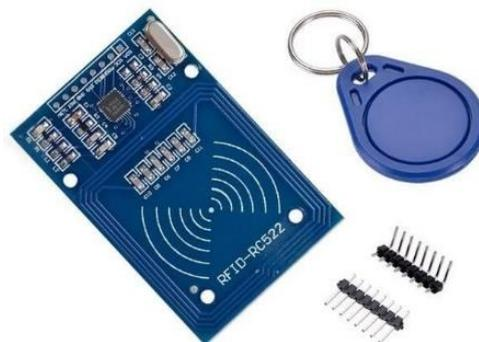
**Gambar 2.9 Modul RFID MFRC522**
