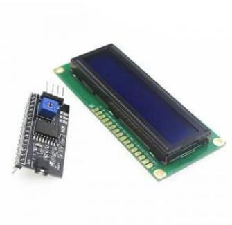
Gambar 2.10 Modul LCD 1602 + I2C Backplate Module
