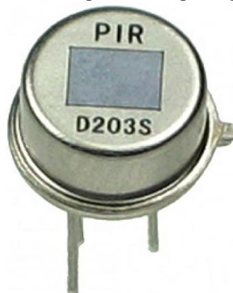
**Gambar 2.11** Pyroelectric sensor
