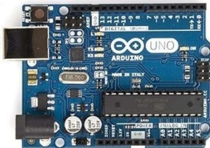
**Gambar 2.4** Papan Arduino Uno
