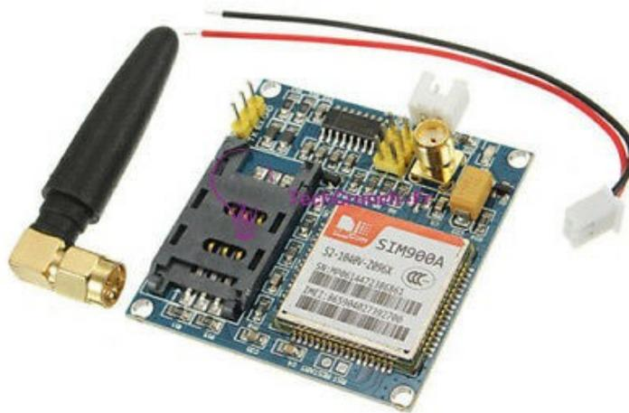
**Gambar 2.6** Modul GSM SIM900A
