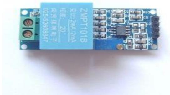
**Gambar 2.14 Sensor Tegangan ZMPT101b**
