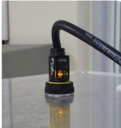
**Gambar 2.20** Ultrasonik Proximity Sensor
