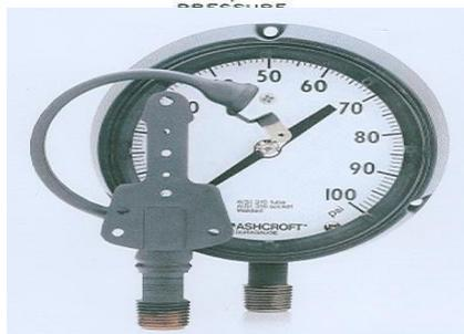
Gambar 2.8 Bourdon Tube (C-type) (Fraden, 1996)
