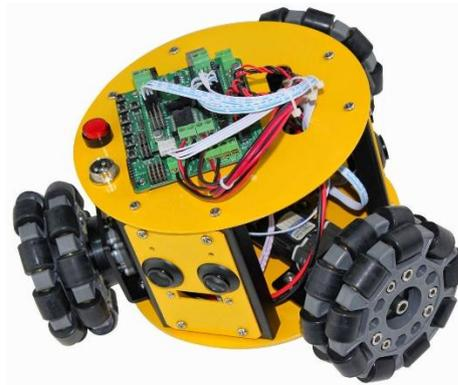
**Gambar 2.2. Robot Beroda Tiga Omni**
