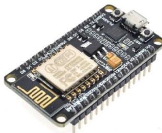
**Gambar 2. 4** NodeMCU ESP8266
