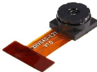
**Gambar 2.10** Sensor Kamera OV 2640
