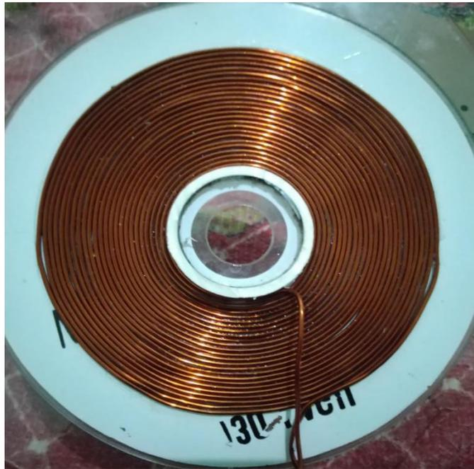
**Gambar 2.19** *Resonant Coil*
