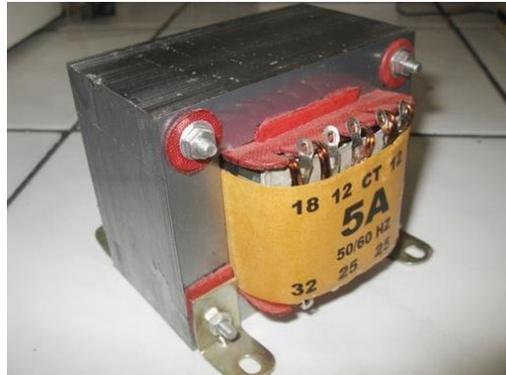
**Gambar 2.8** Transformator *Step-Down*
