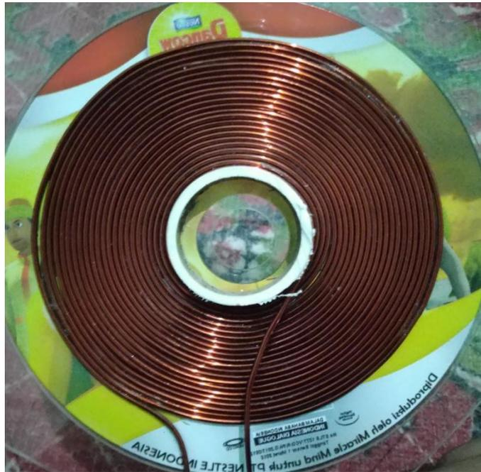
**Gambar 2.17** *Resonant Coil*
