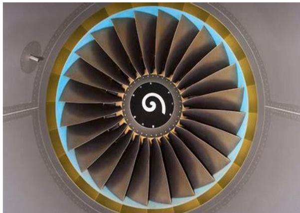
**Gambar 2.5** *Fan Blade* (ASEN 5063 Aircraft Propulsion Final Report, 2015)
