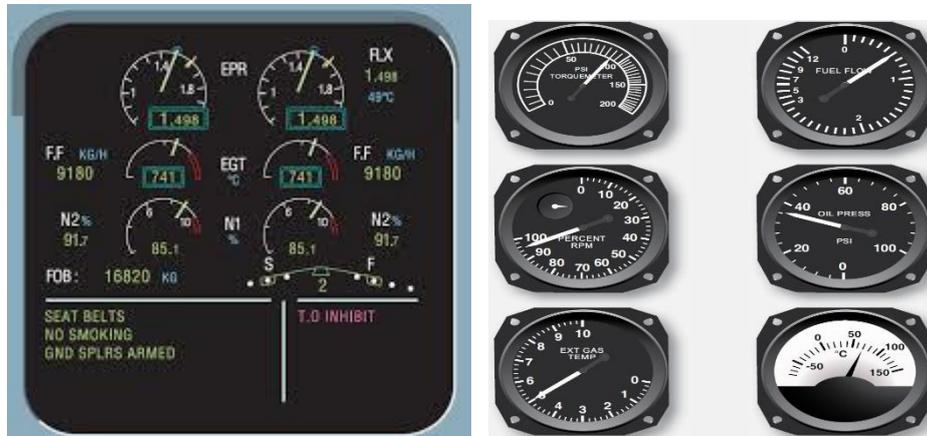
**Gambar 2.1** *Engine Indicating Instrument* (Ira H.Abbot, 2017)
