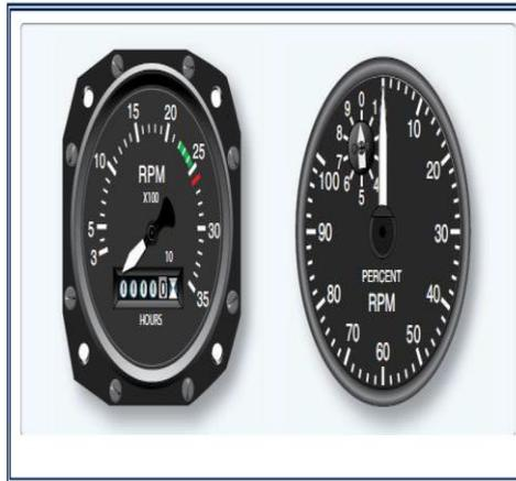
**Gambar 2.2** Tachometer (*Module 20 Aircraft Instruments, 2016*)
