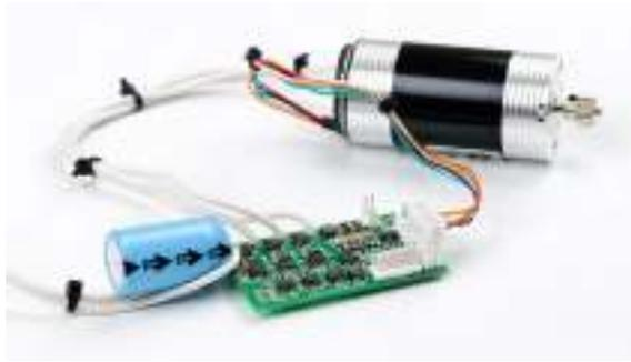
**Gambar 2.4** Modul *motor Controller*
