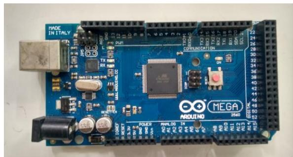
**Gambar 2.5** Arduino Mega 2560
