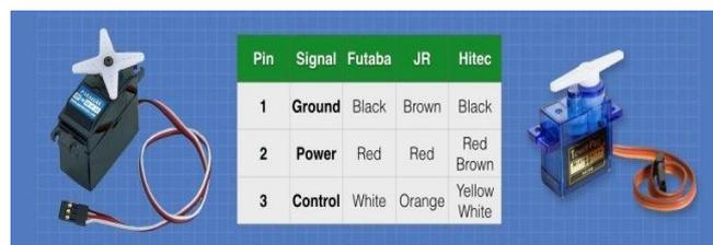
**Gambar 2.9** Connector Motor Servo
