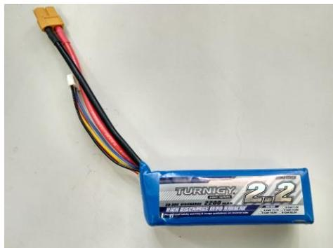
**Gambar 2.12** Baterai LiPo 2200mAh
