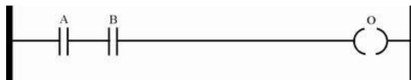
Gambar 2.12 Diagram Rangkaian AND (Nugie, 2008)
