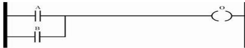
Gambar 2.11 Diagram Rangkaian OR (Nugie, 2008)
