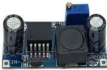
Gambar 2.15 DC Step Down LM2596
