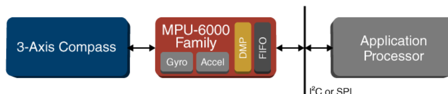
Gambar 2. 6 Diagram Modul MPU-6050
