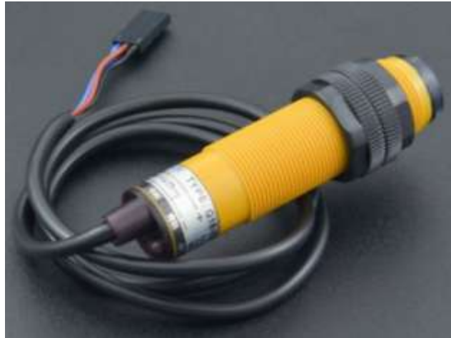
Gambar 2.17 Sensor Infra Red Proximity E18-D80NK [11]
