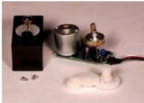
**Gambar 2.8** Sistem Mekanik Motor Servo
