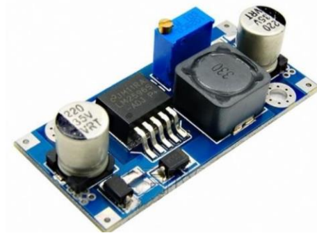
Gambar 2.11 Step down LM2596 [12]
