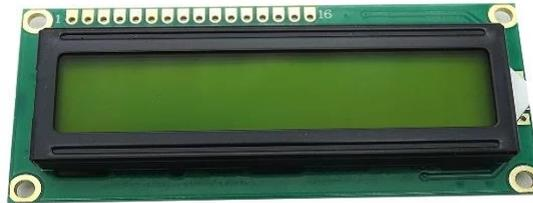
Gambar 2.6 LCD 2x16<sup>[9]</sup>
