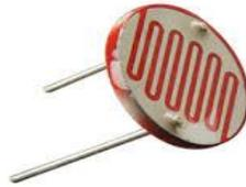
**Gambar 2.12 Light Dependen Resistor**
