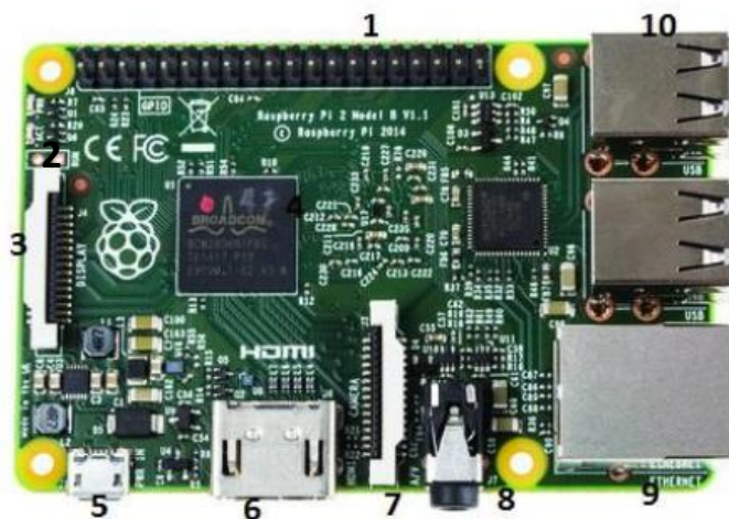
Gambar 2.2 Arsitektur Raspberry Pi 3 Model B [6]
