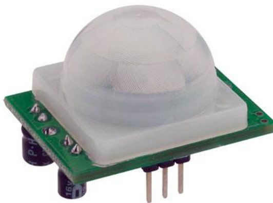
Gambar 2.5. Sensor PIR ( Passive Infra Red ) [9]
