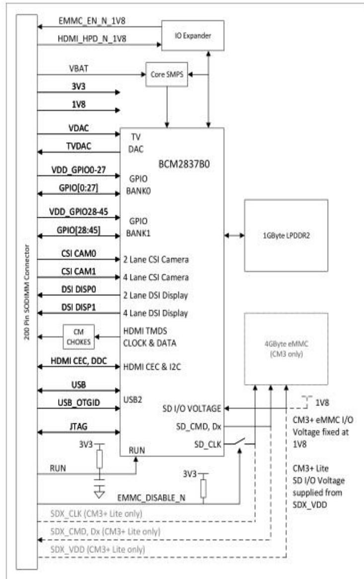
Figure 1: CM3+ Block Diagram
