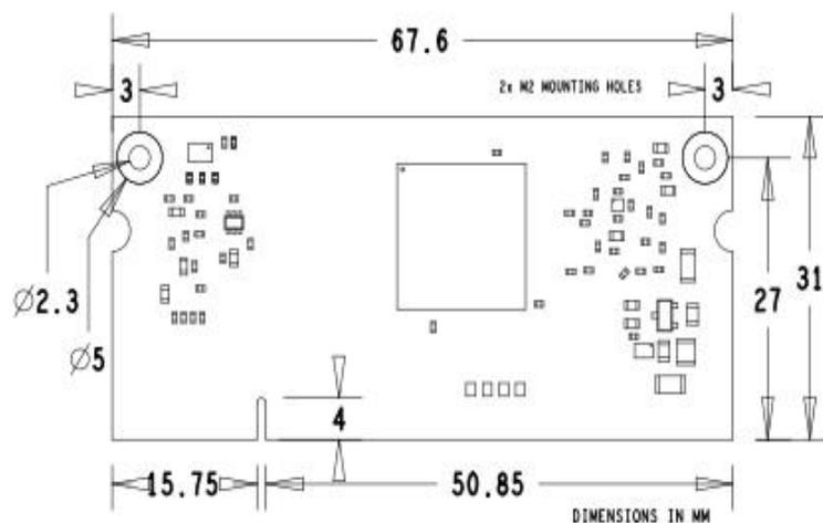
Figure 2: CM3+ Mechanical Dimensions
