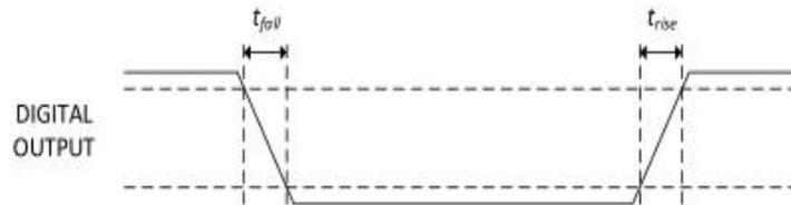
Figure 3: Digital IO Characteristics
