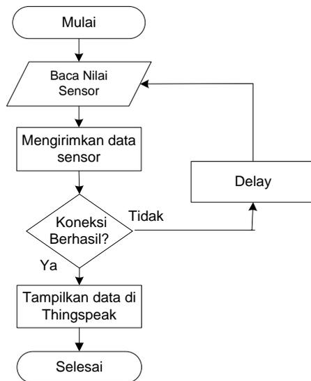
Gambar 4. Diagram Alir Sistem Monitoring
