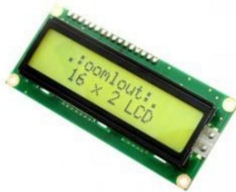
**Gambar 2.4 LCD 16 x 2 [4]**
