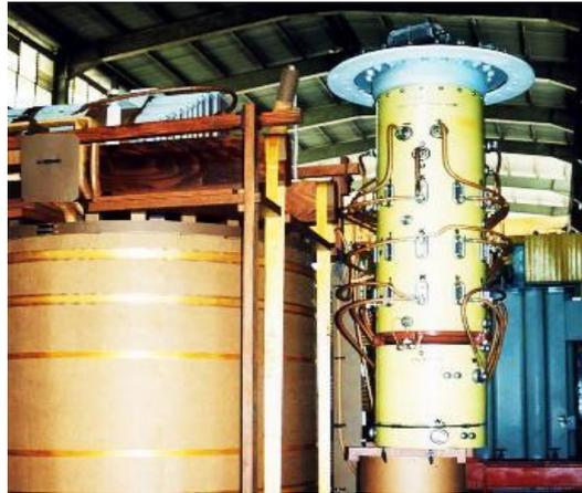
Gambar 2.22 *On Load Tap Changer*<sup>[5]</sup>
