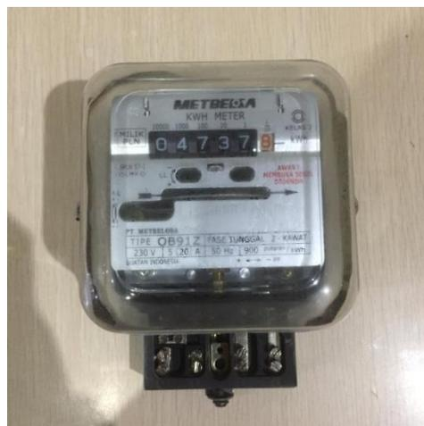
Gambar 2.4 Kwh meter analog
