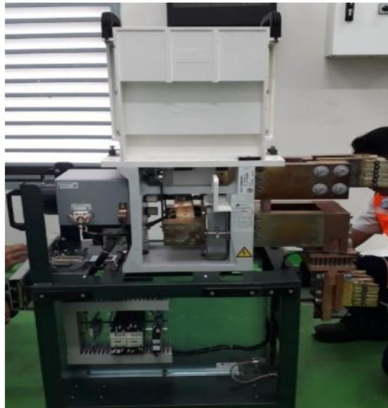
**Gambar 2.7** *High Speed Circuit Breaker*
